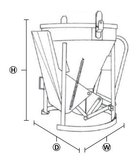
A versatile general purpose skip, with a levered discharge that can be used as a bottom discharge skip for mass concrete pours, or by lowering the side chute can be used as a side discharging skip for more accurate placing of concrete in shutters.
