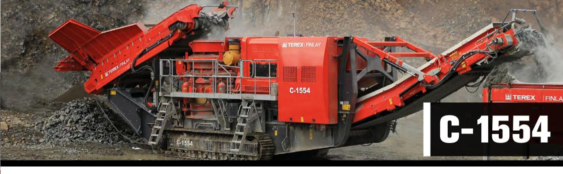
The Terex Finlay C-1554 is the highest capacity machine in the current range of cone crushers. The plant has been specifically developed for quarry operators, construction companies or contractors producing large volumes of aggregates. The plant can accept an all in feed from a primary crusher, excavator or shovel to provide high reduction ratios and produce a product with excellent cubicity.
