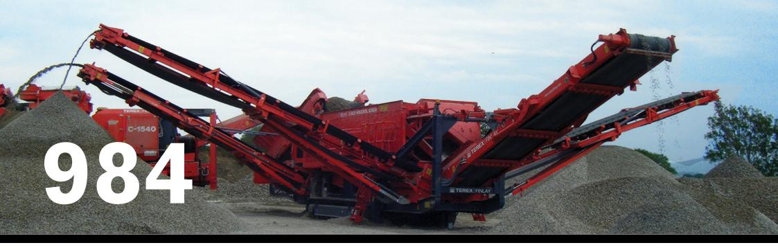
The Terex Finlay 984 is a high performance horizontal 3 deck screener that is easy to set up, versatile and ideal for handling large volumes of material in quarrying, mining and recycling applications.
