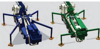
Due to the combination of front X and rear H outriggers the S 34 X can set up without the space hogging footprints of the other outrigging systems.
