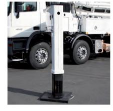
All outrigger cylinders operate in a protective Tube system, so the the cylinders and the piston rods are protected against mechanical damage.
