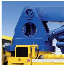
The spacious design of the turret allows good accessibility to the pipeline.
