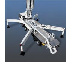
The torsion resistant frame and the far in the rear lying pivot joint assure that the outriggers safely transfer the forces into the ground - the result is outstanding stability.
