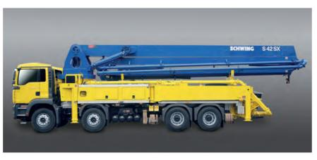
Unlike ordinary concrete pumps the S 42 SX does not need complicated Telescopic or folding outriggers. The SX system allows for rapid and space saving deployment.
