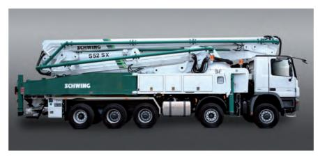
The pumps are designed to distribute the load evenly onto the 5 axles so there is no overhang of the boom package. The pivot point of the rear outriggers is above the first rear axle. This gives the machine a solid stand during pumping operations.
