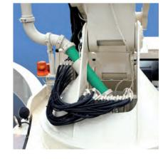
The orderly placement of hydraulic and pipe lines allow good accessibility to the turret.
