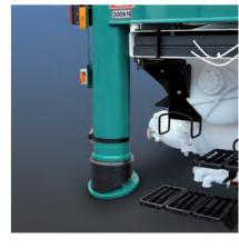
The front and rear outriggers come with attached swivel pads.
