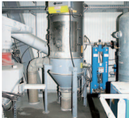
In order to keep the mixing plant's platform free from dust to a large extent, a forced dedusting device can be installed.
