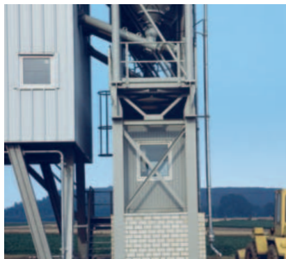
The raised control container with MC control system and high-voltage section allows free sight to the discharge hopper of the mixer.
