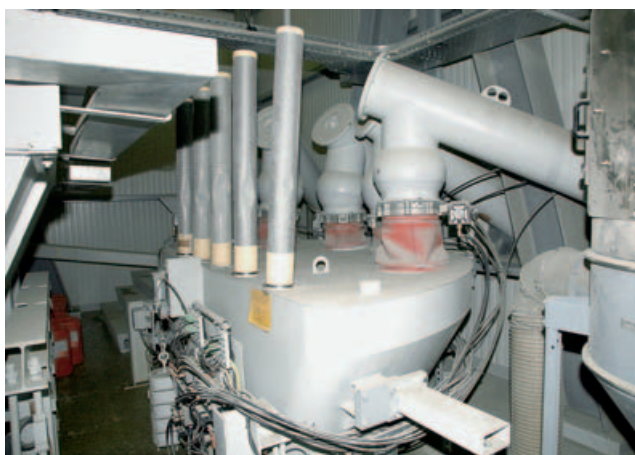
The cement weighing system is equipped with load cells.
