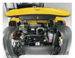
For full access: if the equipment needs to be serviced, the side parts of the rear weight can be removed.
