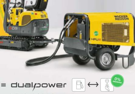
In addition to the existing diesel engine, the compact excavator can be operated emission-free via an electro-hydraulic generator.
