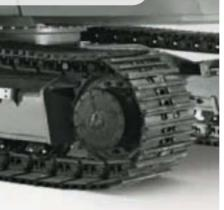
The rubber track: high level of comfort with low noise development and no damage to sensitive subsurfaces.
